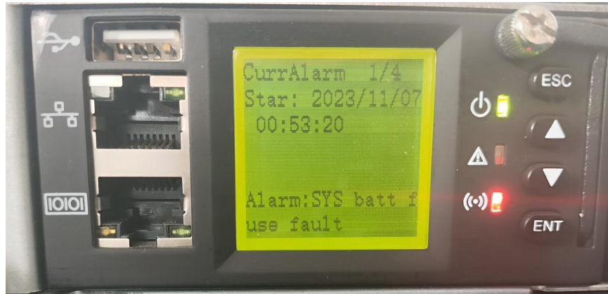
Figure 3-11 Current alarm information screen
