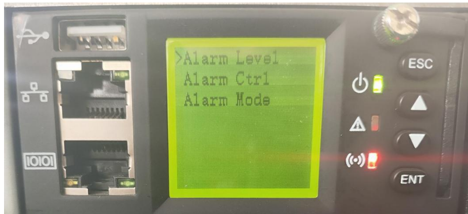
Figure 3-14 Alarm parameter setting screen
