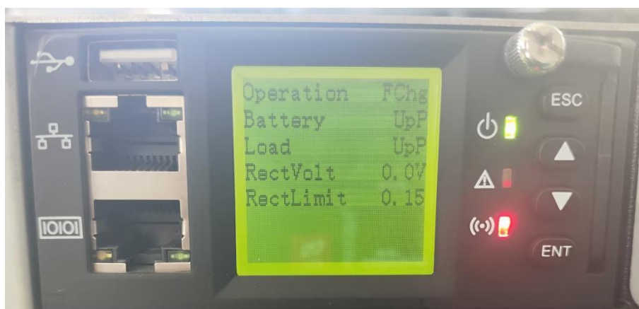
Figure 3-13 Control output screen
