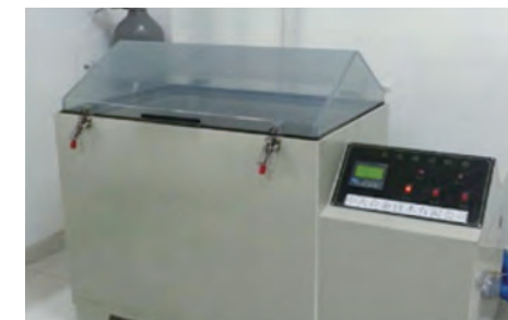
Sulfur dioxide test box
