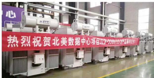
The U.S. data center project was constructed by Northern National Data Center Corporation. Zhongtian Technology provided a complete set of low-voltage power distribution system optimization solution for the project, which is now in operation and provides a strong guarantee for reliable and safe power supply to the data center. 14 SLB-3300/13.8 oil-immersed transformers were supplied.
