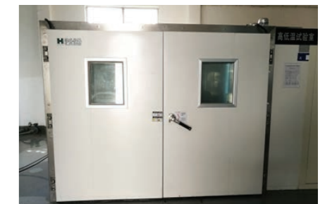
Temperature Cycling Test chamber
