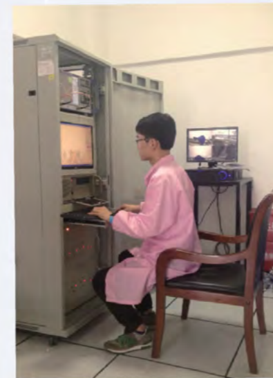
Far field testing system for base station antenna
