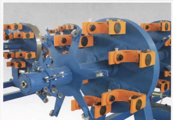
Steel wire armoring cage
